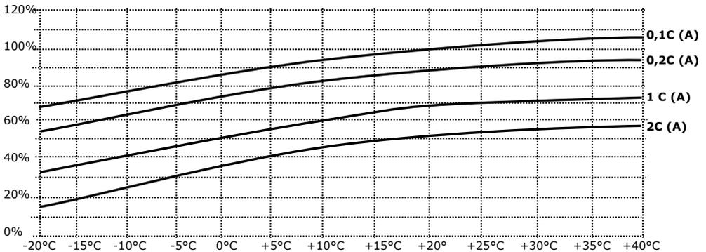
A low temperature reduces remaining capacity.
